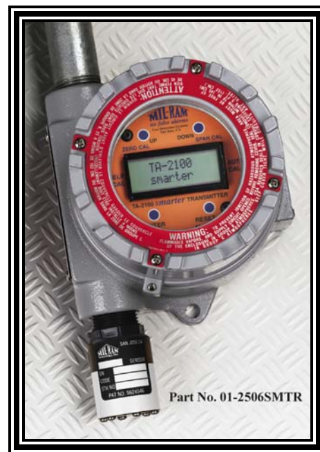
2 line x 12 Character Back-lit LCD Display
