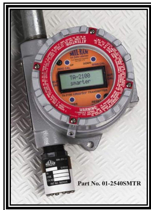
2 line x 12 Character Back-lit LCD Display
